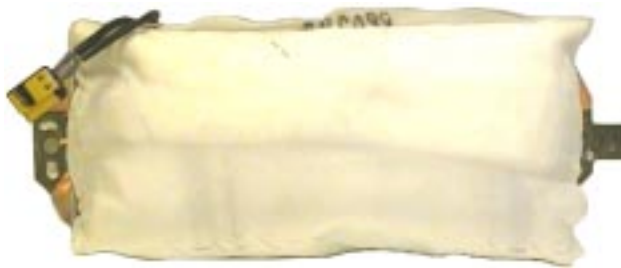
2-Stage Passenger Airbag (Front View)
